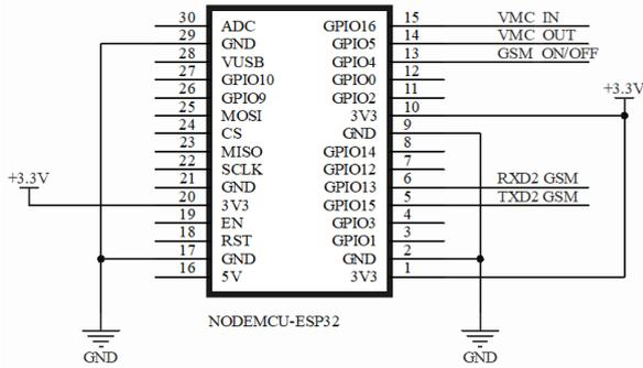
Fig. 7. NODEMCU-ESP32 modules.
