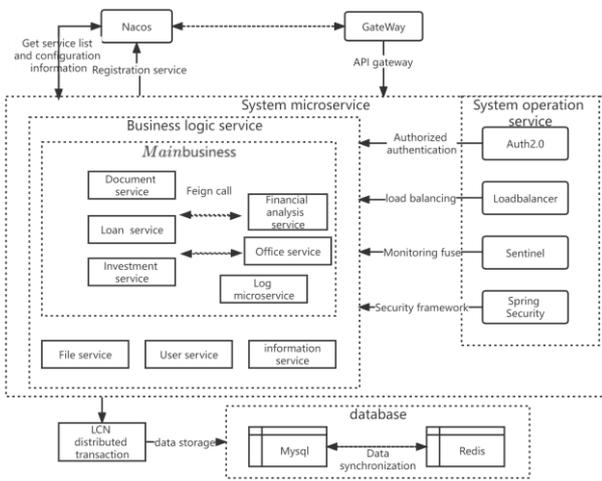
Fig. 3. Overall system architecture.
