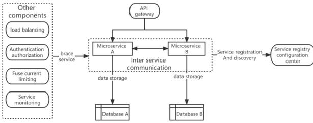
Fig. 2. Microservice architecture.
