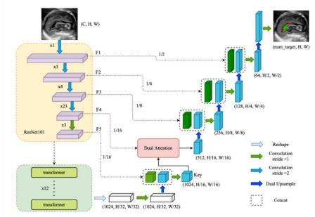
Fig. 3. The structure of the proposed network.
