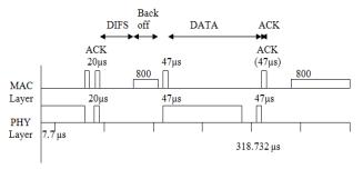
Fig. 3. Data Exchange of IEEE 802.11 Standard.
