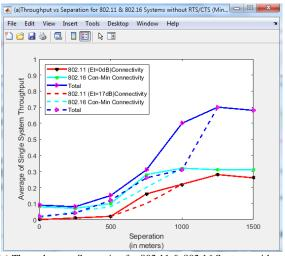
(a) Throughput vs Separation for 802.11 & 802.16 Systems without RTS/CTS (Minimum connectivity)
