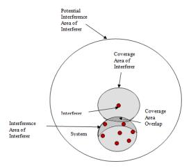
Fig. 1. Coexistence system geometrical model.
