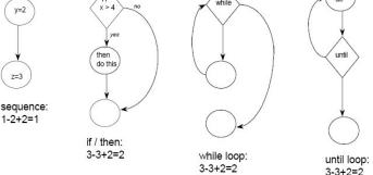
examples of calculations for the cyclomatic complexity for four basic programming structures. Fig. 3. Cyclomatic Complexity for different types of structures (source: [16]).
