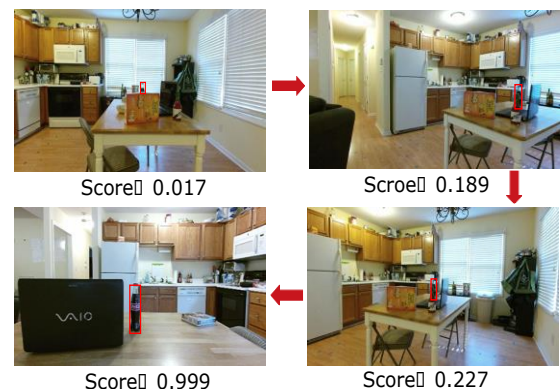
Fig. 1. The robot moves in the scene, changes the view, and the classifier's score for the object changes. When the object gets high score, it can be well detected.
