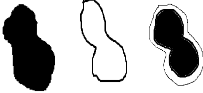
Fig. 1. (a) Binary image, (b) Dilation result, and (c) Erosion result.
